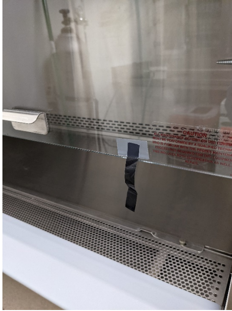
{The tape provides a quick visual of air flow inward.}
