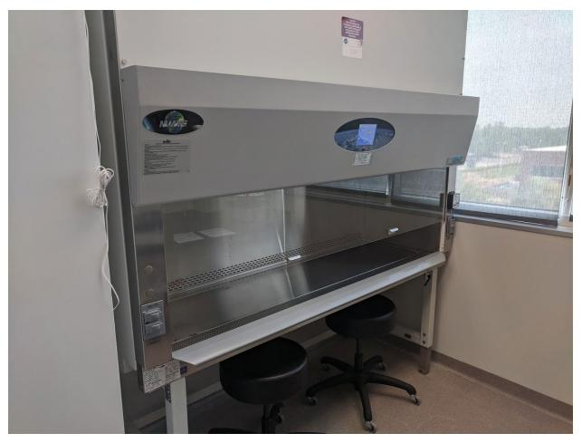
{B2 biosafety cabinets exhaust 100% of the air to the outside. UPHL has several.}
