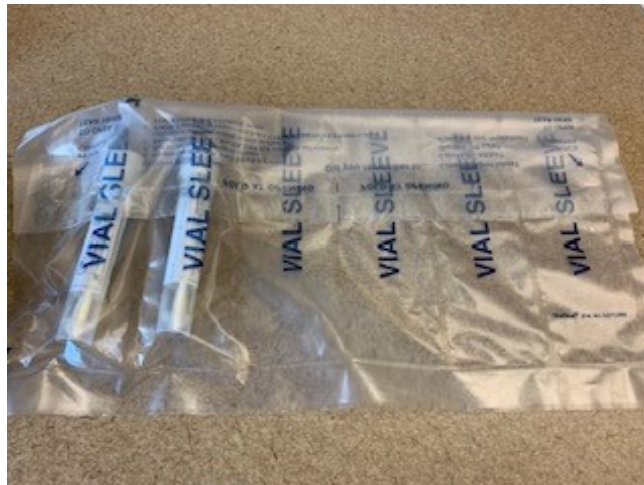
Individual eswabs sealed in separate compartments of vial sleeve
